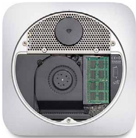
Earlier versions of the Mac mini made RAM upgrades a difficult process for the DIYer. Apple frowned on cracking open the early Mac minis, and I do mean cracking open. Special tools were required to pry the two halves of
